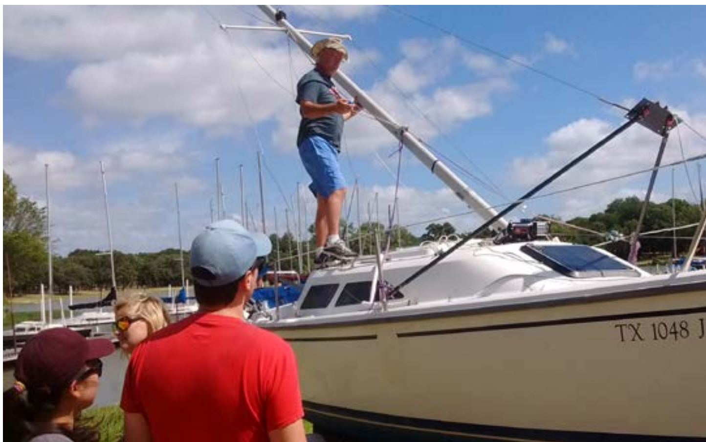
Jeff Owen's family watches as he single-handedly raises the mast on his Catalina 22. Jeff refused any assistance because he wanted to try out his 12 volt power winch and A-frame. The winch features a hand-held remote and not only did he get the job done, he made it look easy!
